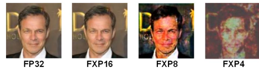
Fig. 2. Difference in generated image quality based on the datatype
