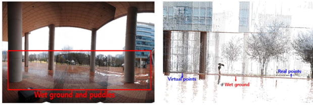
Fig. 10. Reflection on non-glass surface. The virtual points are generated by the reflection on the puddles and wet ground in a rainy day.
